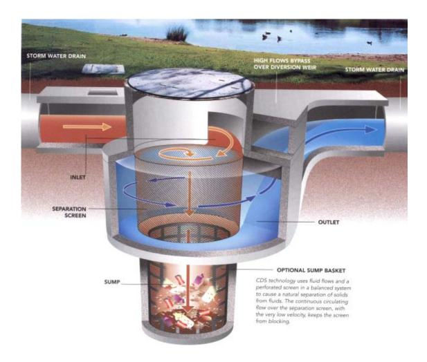
Figure 2-1. Schematic Diagram of CDS Unit.
