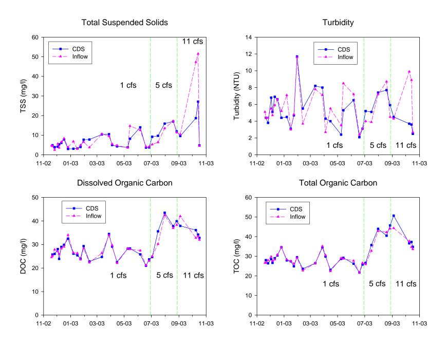
Figure 5-18. Concentrations of TSS, Turbidity, DOC and TOC in Inflow and Outflow of the CDS Unit.
