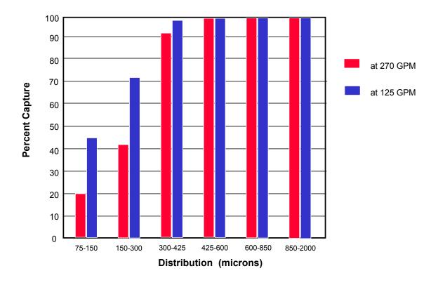
Figure 2-2. CDS Unit Particle Capture vs. Flow Rate (1200 micron screen).
