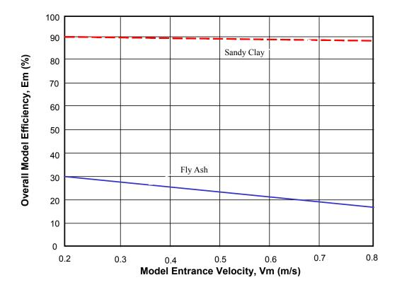
Figure 2-5. FIT Study Overall Removal Efficiency vs. Flow Rate.
