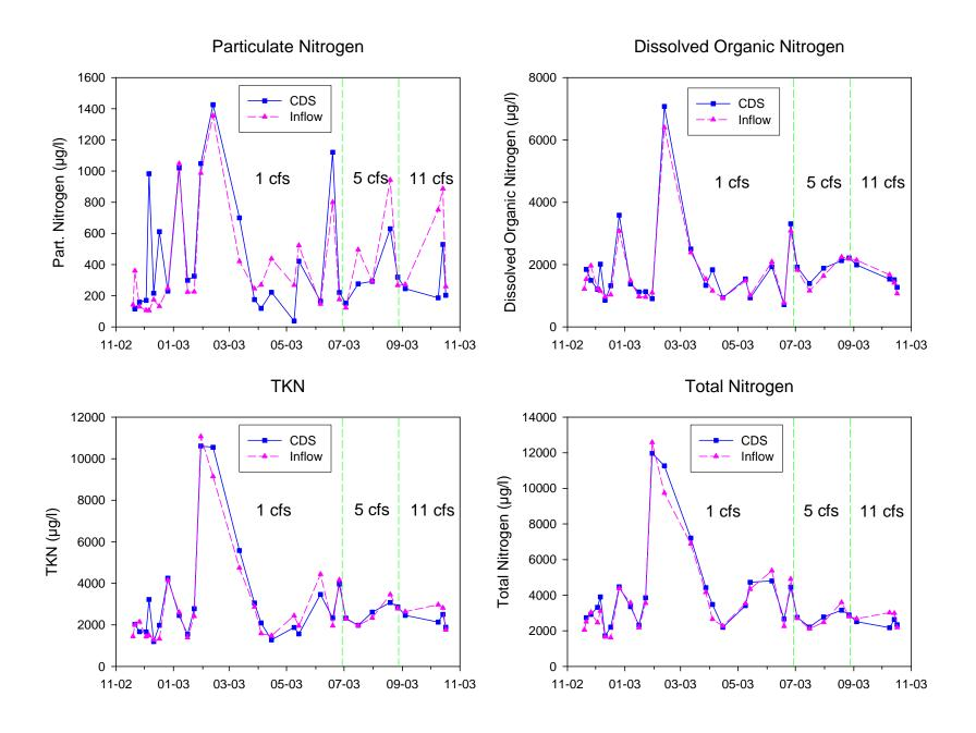
Figure 5-17. Concentrations of Nitrogen Species in Inflow and Outflow of the CDS Unit.
