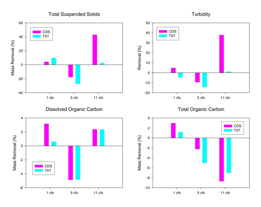
Figure 5-24. Comparative Mass Removal Efficiencies for TSS, Turbidity, DOC and TOC in the CDS and TST Units.
