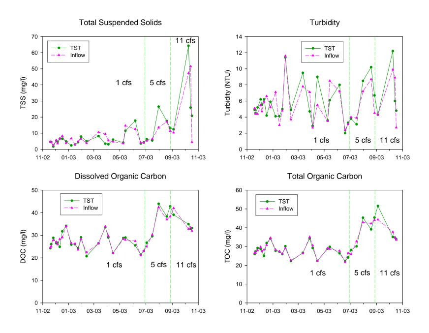
Figure 5-21. Concentrations of TSS, Turbidity, DOC and TOC in Inflow and Outflow of the TST Unit.
