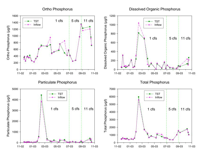
Figure 5-19. Concentrations of Phosphorus Species in Inflow and Outflow of the TST Unit.
