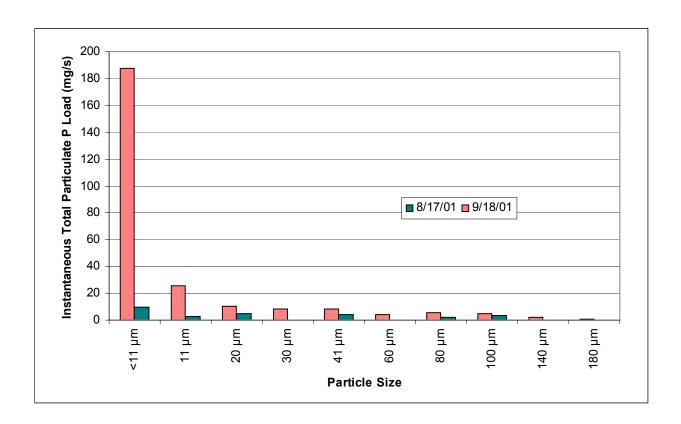
Figure 4-2. Lettuce Creek Instantaneous Total Particulate Phosphorus Load by Particle Size.
