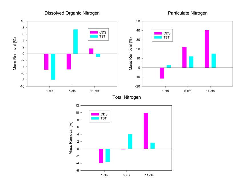
Figure 5-23. Comparative Mass Removal Efficiencies for Nitrogen Species in the CDS and TST Units.
