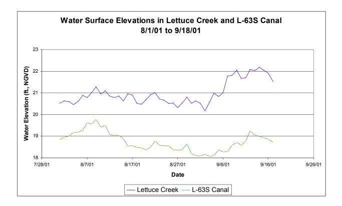
Figure 3-2. Plot of Recorded Water Surface Elevations in Lettuce Creek and L-63S Canal.
