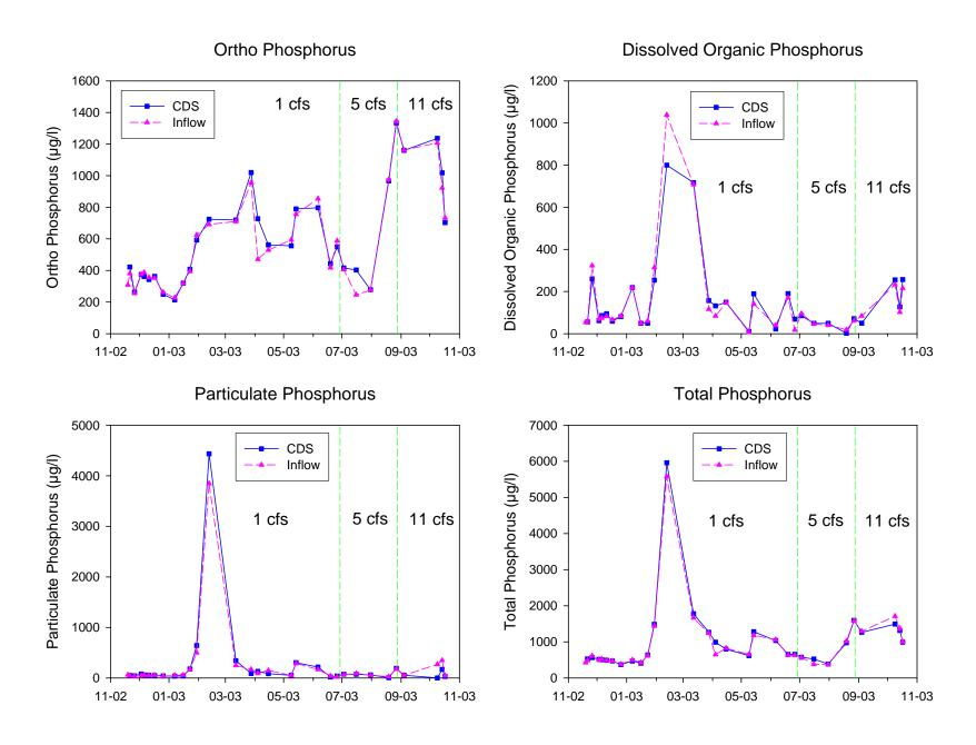
Figure 5-16. Concentrations of Phosphorus Species in Inflow and Outflow of the CDS Unit.
