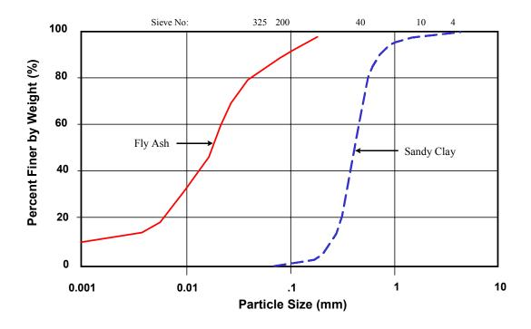
Figure 2-4. Grain Size Distribution Curves for FIT Study.
