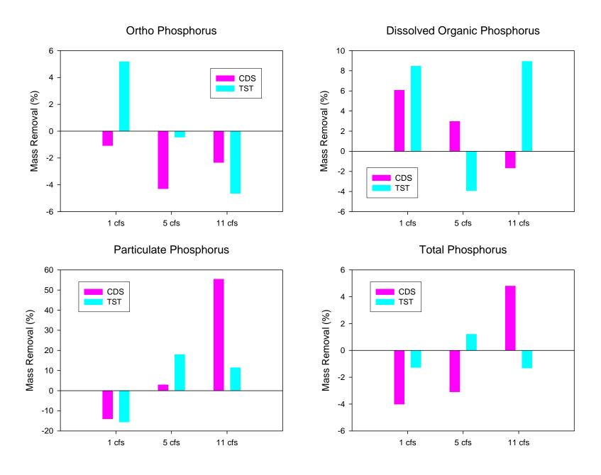
Figure 5-22. Comparative Mass Removal Efficiencies for Phosphorus Species in the CDS and TST Units.
