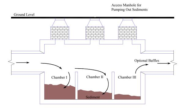
Figure 2-3. Schematic Diagram of Sediment Trap.
