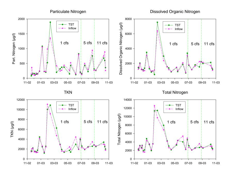
Figure 5-20. Concentrations of Nitrogen Species in Inflow and Outflow of the CDS Unit.
